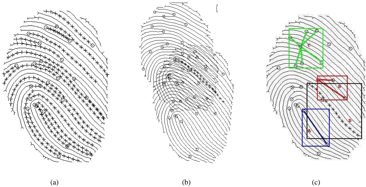
Fig. 5. Ridge similarity: (a) minutiae and associated ridges (represented by points sampled at average inter-ridge distance), (b) false alignment with similar ridge pair (beyond the tolerance of an adaptively compensating minutiae matching algorithm), and (c) region sizes of local similarity models of three minutiae matchers: A(lower left blue box): Bozorth minutiae pair, B(small red box): triplet model [3], C(top green box): k-minutiae model. D(black): labels a ridge.
