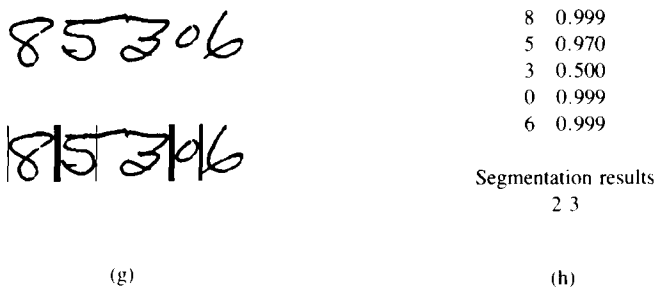
Fig. 18. Cont'd. Steps in processing a handwritten address (second example). (g) Second ZIP Code candidate and its segmentation. (h) digit recognition results of second ZIP Code candidate shown as pairs (recognized digit, confidence).
