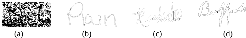
Fig. 7. (a) Noise in the image could not be removed; (b) segmentation method described in the paper failed; (c) broken contours could not be joined during the smoothing process; and (d) the ascenders of the ‘f’ were not picked.
