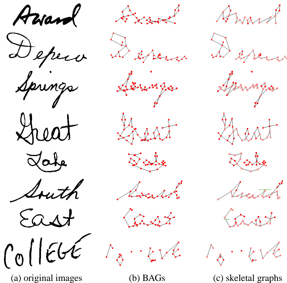
Figure 3.8.1: Examples of skeletal graphs on real-life images. Truths from top down: Award, Depew, Springs, Great, Lake, South, East, College.
