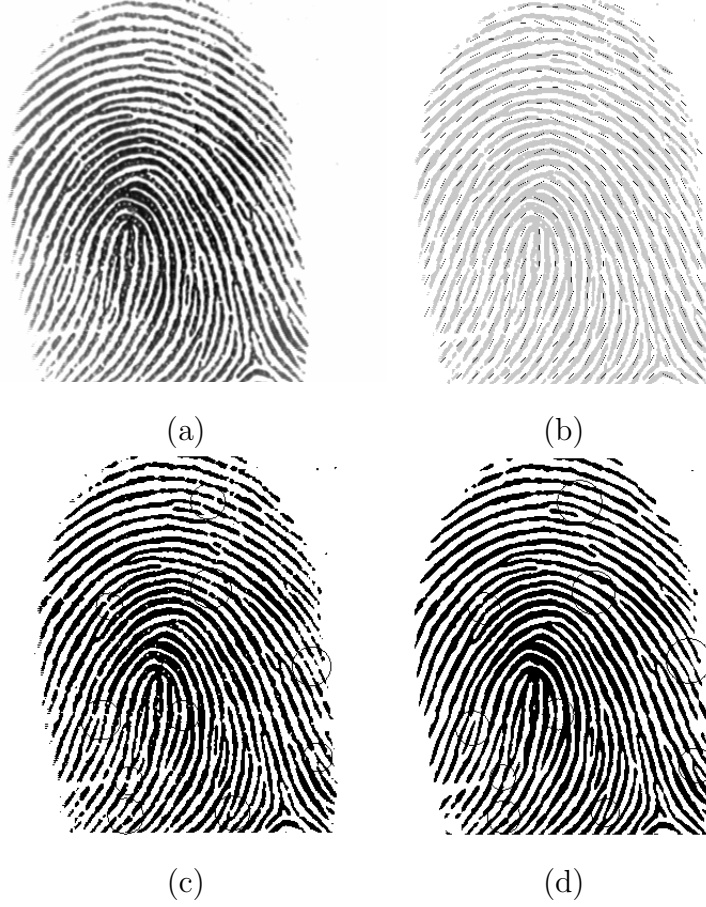
Fig. 7. (a)Original Fingerprint image. (b)orientation field. (c)The binarization of filtered image by Anisotropic filter. (d)The binarization of filtered image by the proposed filter.
