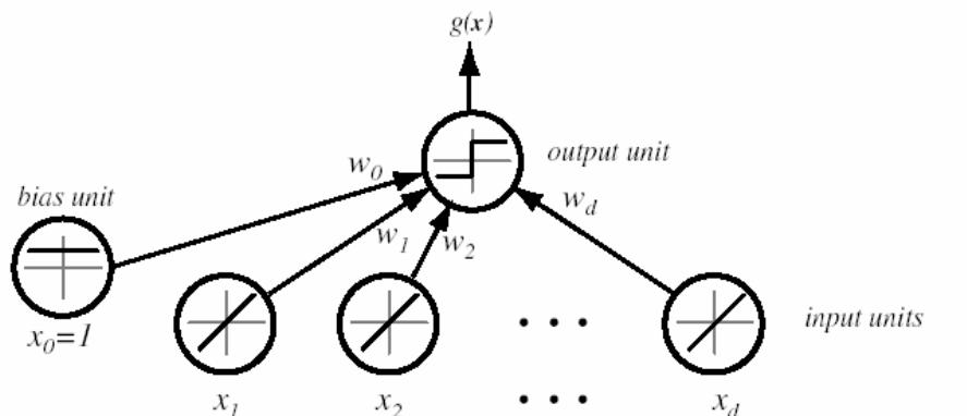
Each unit is shown as having inputs and outputs. The input units exactly output the same values as the inputs (except the bias unit which outputs a constant 1). The output unit emits a 1 if the sum of its weighted inputs is greater than zero and -1 otherwise
