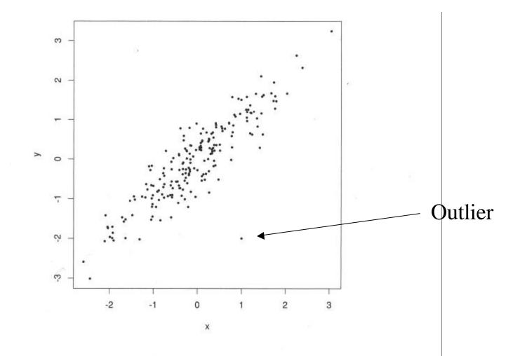
**Figure 2.6** A plot of 200 points from highly positively correlated bivariate data (from a bivariate normal distribution), with a single easily identifiable outlier.
