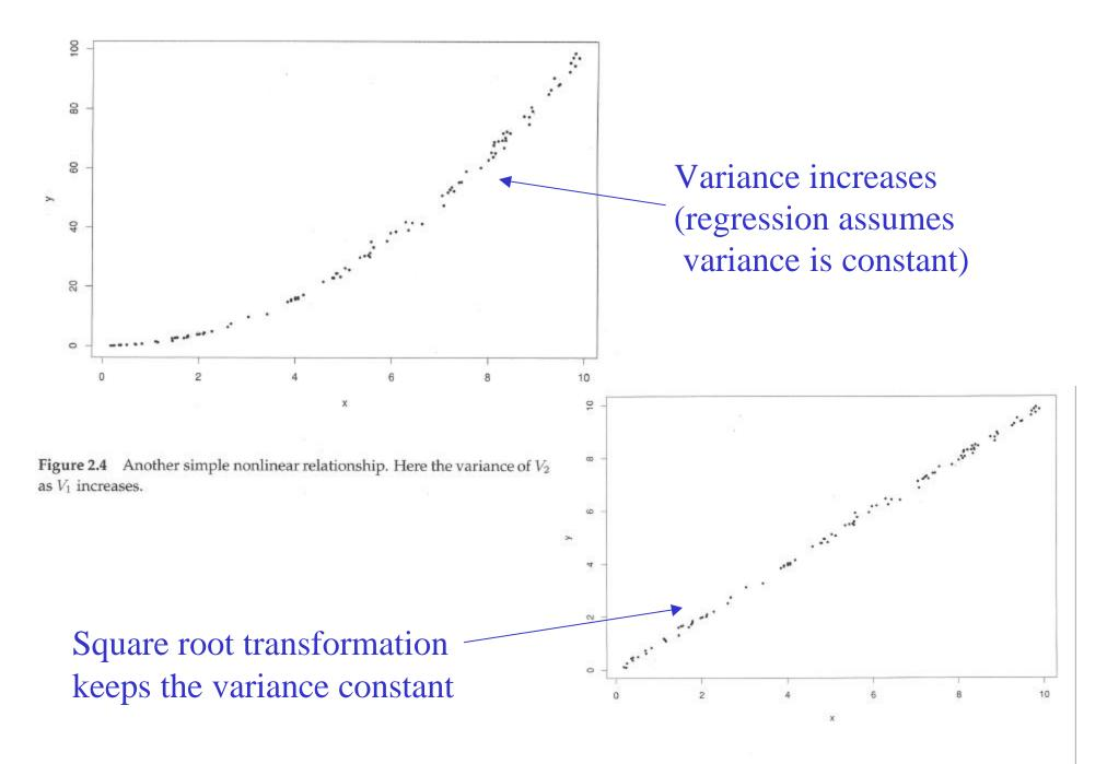
**Figure 2.5** The data of figure 2.4 after a simple square root transformation of  $V_2$ . Now the variance of  $V_2$  is relatively constant as  $V_1$  increases.
