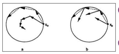
(a) Without teacher forcing, trajectory runs astray (solid lines) while the correct trajectory are the dotted lines
