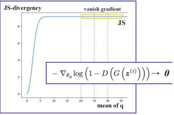
When D is perfect, we are guaranteed with  $D(x)=1, \forall x \in p_r$  and  $D(x)=0, \forall x \in p_g$ Therefore loss L falls to zero and there is no gradient to update L during learning Figure below: when the discriminator gets better, the gradient vanishes fast
