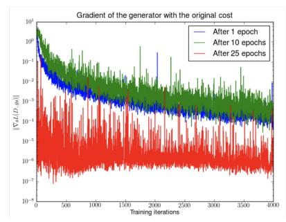
First, a DCGAN is trained for  $1,\,10$  and 25 epochs. Then, with the G fixed, D is trained from scratch and measure the gradients with the original cost function
