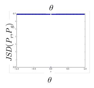
EMD is continuous and provides a usable gradient JSD is discontinuous and there is no usable gradient
