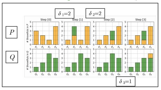
Move 2 units from  $P_1$  to  $P_2 \rightarrow (P_1, Q_1)$  match Move 2 units from  $P_2$  to  $P_3 \rightarrow (P_2, Q_2)$  match Move 1 unit  $Q_3$  to  $Q_4 \rightarrow (P_3, Q_3)$ ,  $(P_4, Q_4)$  match
