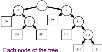
chooses to send the input example to the child node on the left (0) or the child node on the right (1). Internal nodes are circles Leaf nodes are squares.
