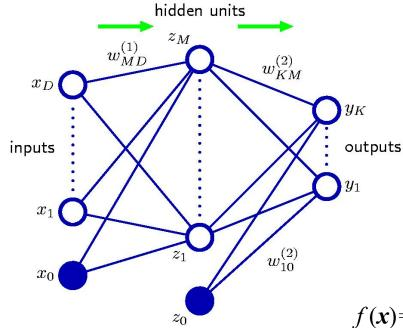
*K* outputs  $y_1, ..., y_K$  for a given input *x* Hidden layer consists of *M* units
