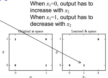
When  $h_1=0$ , output is constant 0 with  $h_2$
