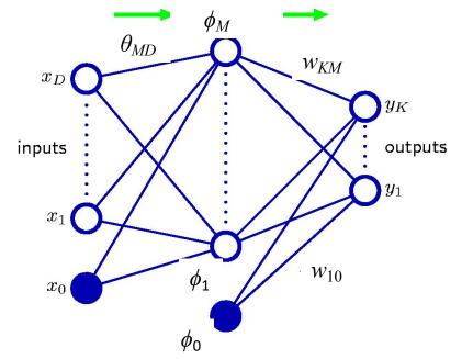
*K* outputs  $y_1, ..., y_K$  for a given input *x* Hidden layer consists of *M* units
