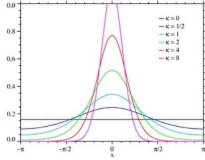
Figure 1. Von-Mises distribution PDF
