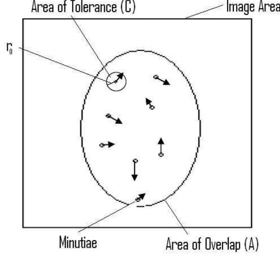
Fig. 8. Graphical representation of the Pankanti matching algorithm. Input print overlaps the template fingerprint. Minutiae are matched based on the location and orientation tolerance
